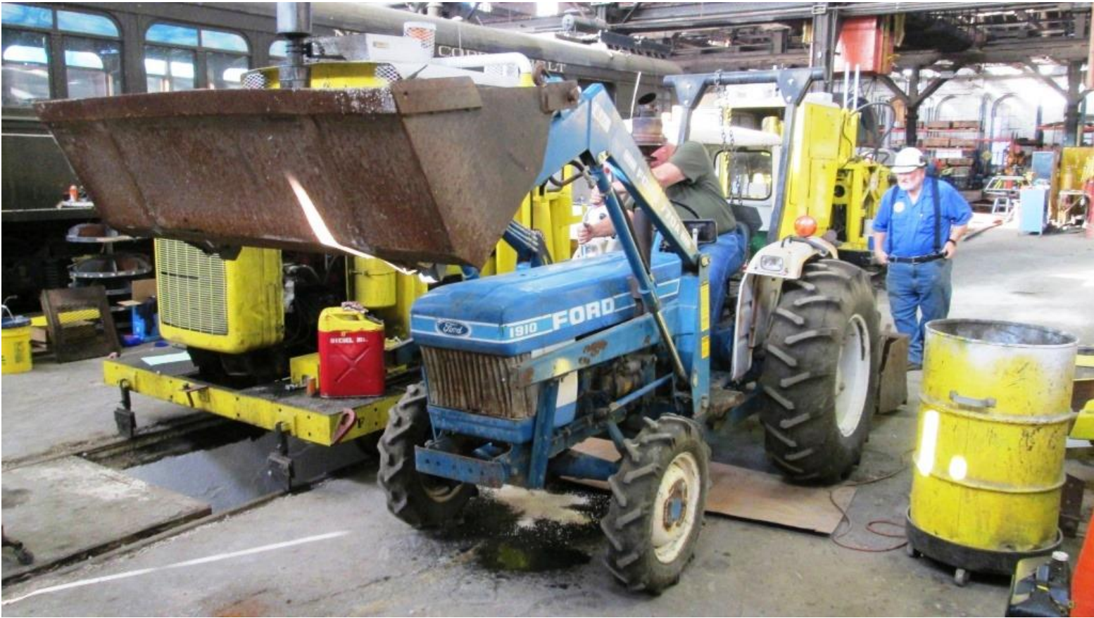
With the tractor now fully functional, Gene tests the hydraulics by lifting the bucket
