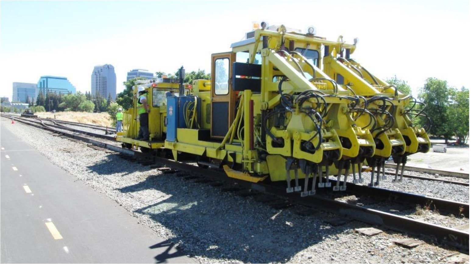
Hospital train: the Kalamazoo tug tows the tamper back into town
