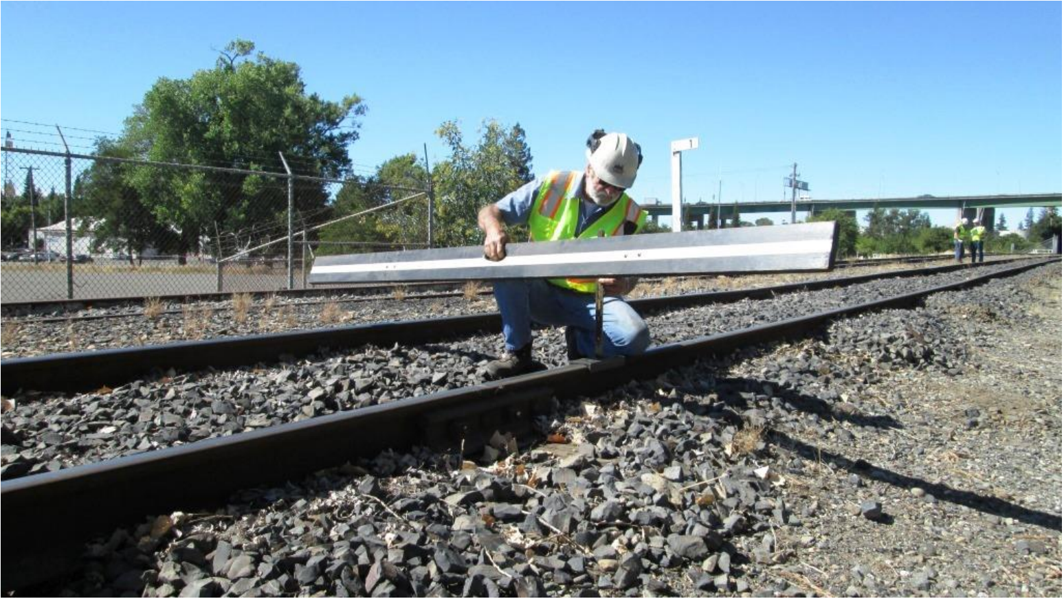
Alan sets up the spot-board and places it on the rails
